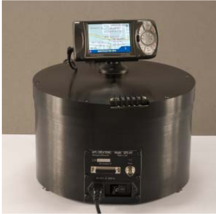
GPS-RT shown above with a typical mobile GPS display unit installed for testing.
