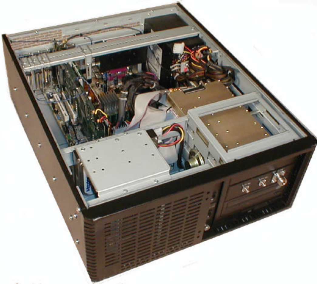
Figure 1 – GPSSIM14 Shown With Top Cover Removed
