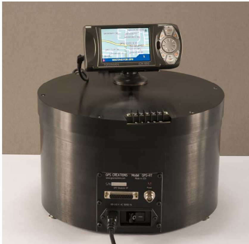
Figure 2 - GPS-RT w/GPS Receiver for Testing
